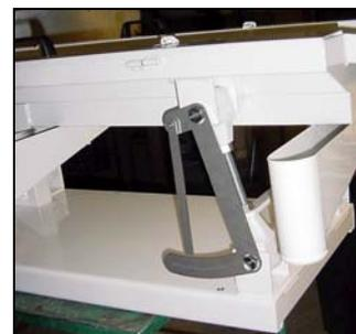
Tool for measuring the angle of the spring inclination
