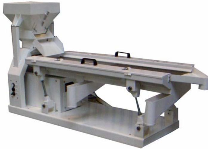
**The LA-VBS precision sizer for laboratory use is designed for grain samples where the kernels are to be graded according to thickness**
